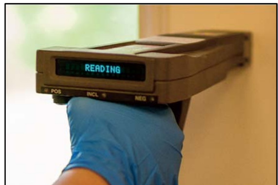
Testing for lead in paint
